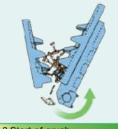
2 Start of crush The remaining material which is larger than the occlusion of the blades is crushed.
