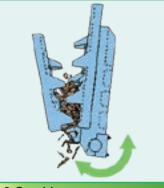
**3** Crushing The continuous crushing action of the blades allows crushed material to drop through.
